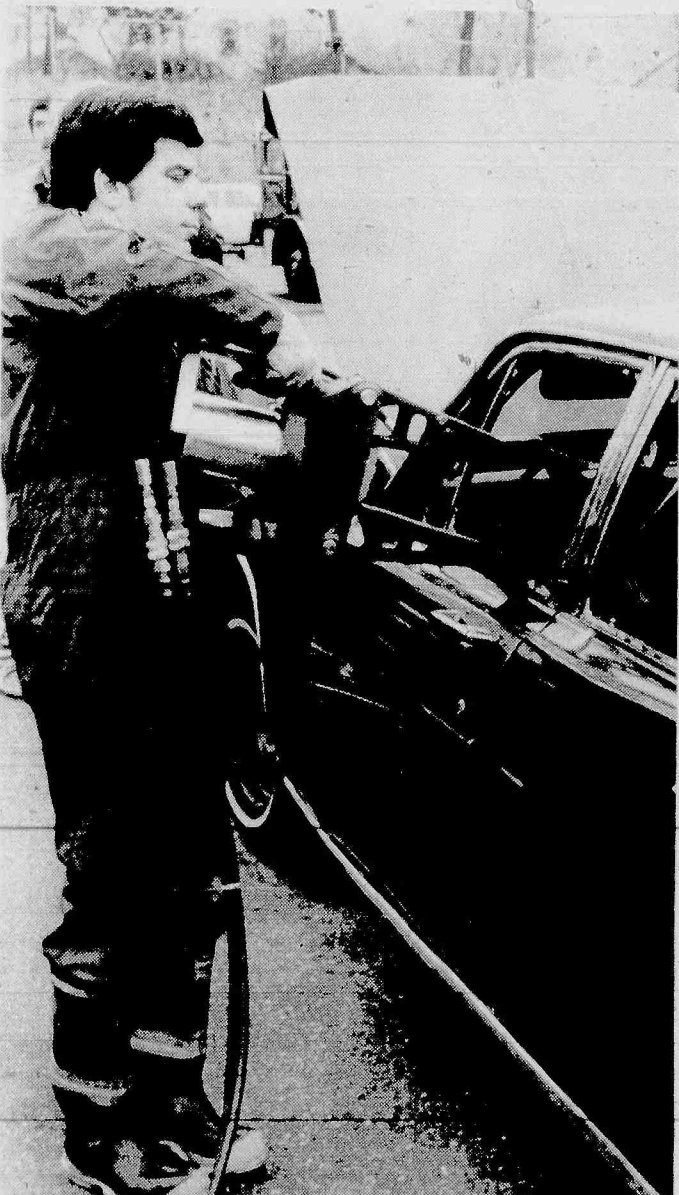
Open Wide — The Lucas Tool is designed to expand parts of the wrecked automobile by spreading the metal apart. Therefore making it easier for rescue teams to reach injured automobile passengers.
